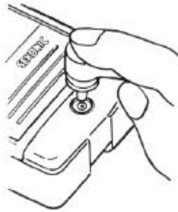
(5) The appropriate F-stop value is displayed on the meter (Fig. 18). For repeat measurement, press the measuring switch again.
