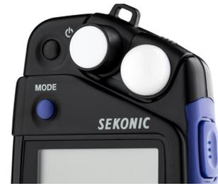
Slide the built-in lumisphere to the right and insert the lumidisc (optional) into the slot over the light receptor lens to measure flat subjects or lighting contrast with precision.
